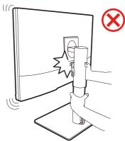
The cable management hole is designed to route the cables and cannot support the weight of the monitor. Never try to lift the monitor by the cable management hole.
